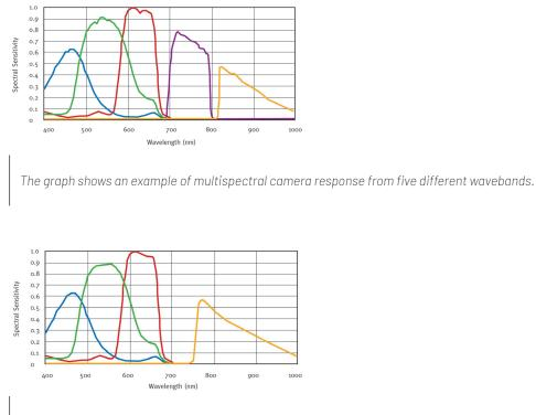
The graph shows an example of multispectral camera response from four different wavebands.
