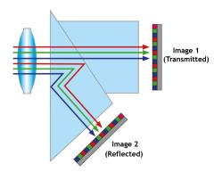
This is another multispectral imaging technique using a beam splitter. In this method, all the optics including the lens are common for both the sensors, unlike the previous method which uses two individual cameras with individual lenses but a common beam splitter.
