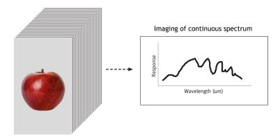
Hyperspectral imaging provides a continuous range of spectra.
