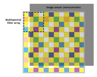
With snapshot mosaic sensor based cameras, it is possible to acquire a multispectral image in one shot. However, multispectral demosaicing is a challenge due to sparse sampling of spectral bands in the filter array.
