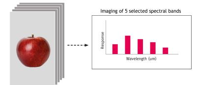
Multispectral imaging consists of spectral bands which are discretely positioned from each other. In other words they do not provide a continuous spectrum.
