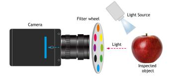
A multispectral camera using filter wheel captures multi-spectral images. This is done by rotating the filter wheel mounted in front of the lens or in-between the sensor and the lens.
