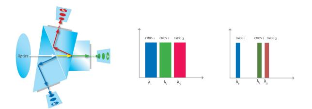
In prism-based cameras, the prism blocks consist of hard dichroic coatings which are interference filters by nature. These filters are responsible for the primary separation of incoming light.
