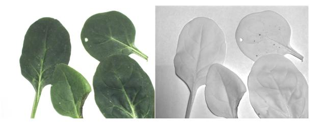
Using multispectral inspection techniques can reveal unwanted dirt particles (see the NIR image), and help to ensure the right quality of spinach leaves before they are packed.
