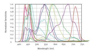
The graph shows an example of multispectral camera response from twelve different wavebands. Source: C. Godau et. al; Evaluation of a multispectral camera system for inline color measurement, Proceedings of the 19. Workshop on Color in Image Processing, Berlin, ISBN: 978-3-942709-08-8
